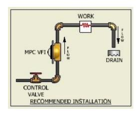
The above diagram shows preferred installation to achieve maximum performance by mounting the VFI in vertical plane between a control valve and drain.
