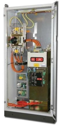
Control fitted into a sheet steel enclosure with circuit breaker, 24 VDC air valve power supply, appropriate line fusing, safety covers, and water-cooled MFDC Inverter Module. Optional hand-held pendant.
