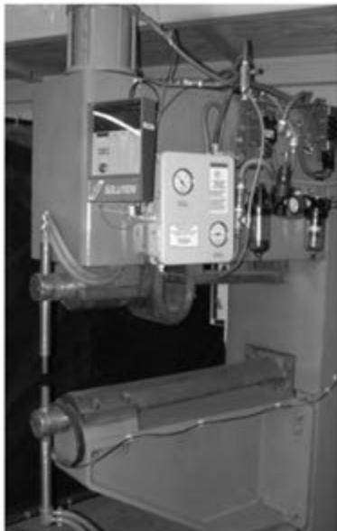
SOFT TOUCH installed on a 200KVA press welder
