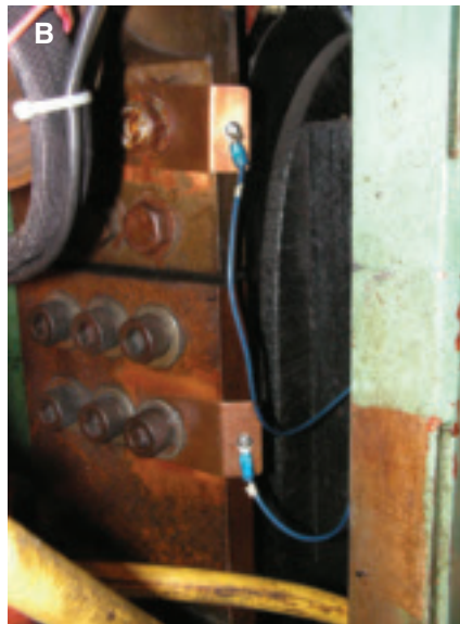
Fig. 6 — A — This system from Unitrol Electronics provides passive electrode pinch-point protection at Ada Metal Products, Inc., Lincolnwood, Ill. B — continuity measuring wires connected to welding transformer secondary pads; C — padlocked NEMA-4 enclosure with precision regulators supply pressure to new solenoid and quick exhaust valves. This arrangement counterbalances an 160-lb ram to less than 40 lb.
