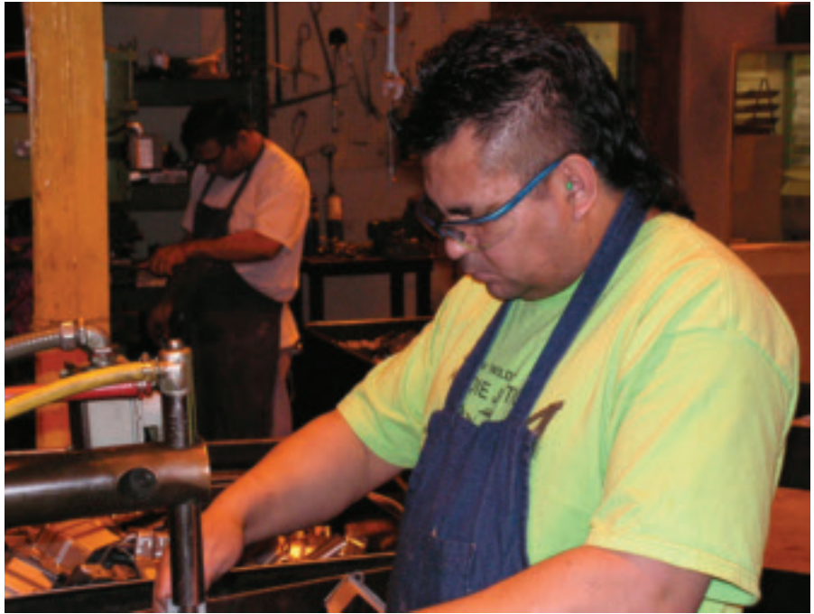
Fig. 2 — Wearing of approved safety glasses with side shields is mandatory for eye protection.
