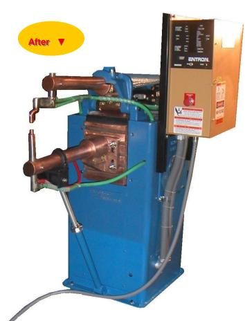
When re-manufacturing Rocker Arm Welders, we look critically at eight main components of the welder: the **frame**, the **bushings/bearings**, the **transformer**, the **pneumatics**, the **secondary**, the **cooling system**, the **weld control/initiation**, and the machine **testing/debugging**. You receive the same quality work you have come to expect from us, along with a warranty to ensure the remanufactured Rocker Arm Welder works as expected.
