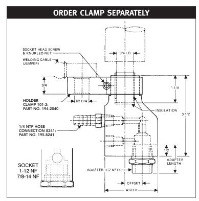
To determine distance adapter sticks out from holder, deduct 1/2-in from length of adapter selected. Water tubes 1/2-in. longer than adapter will install approximately flush with adapter face.
