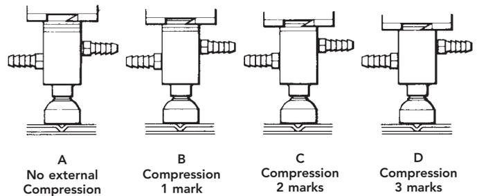
For every one-eighth of an inch that a fast-follow-up is compressed when setting up, a known amount of force is provided, to quickly follow up any reduction in work thickness. Example: at position B, a type MH spring would delivery 310 lb, at C, 440 lb, etc.
